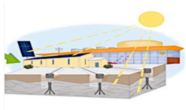
Geoenergy plant at Karlstad University. Illustration by Akademiska Hus.
